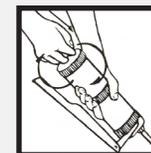
6. To eliminate air bubbles, pull the lever to its out most possible, and push the rod into the tank.
